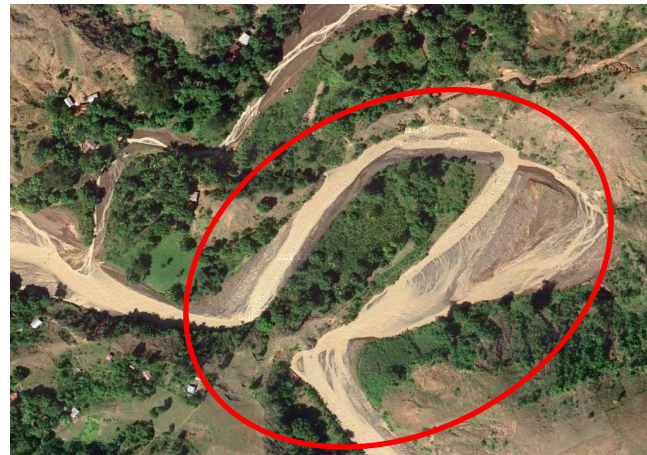
Figure 11: A location of a maximum shear stress (upper reach)
